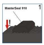
For normal joints width of 200-400 mm, place the waterbar along the middle of the joint. On wide joint surfaces (greater than 100 cm), two parallel waterbars may be laid for added safety.
