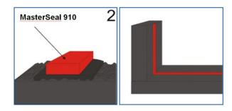
It is important to leave the minimum coverage from both the edges of concrete to provide sufficient concrete cover to absorb the swelling stresses.
