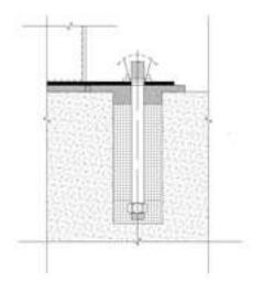
Pouring should be from one side of the void to eliminate any air or presoaked water becoming trapped under the base plate. It is advisable to pour the grout across the shortest distance of travel. The grout head must be maintained at all times so that a continuous grout front is achieved.
